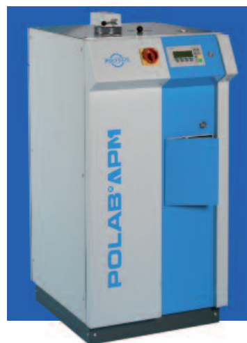
Semi-automatic pneumatic delivery receiving station with magazines for received and empty capsules.
