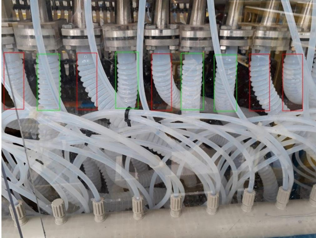
Fluid flow detection for the autonomous plant start-up challenge. Image credit: thyssenkrupp
